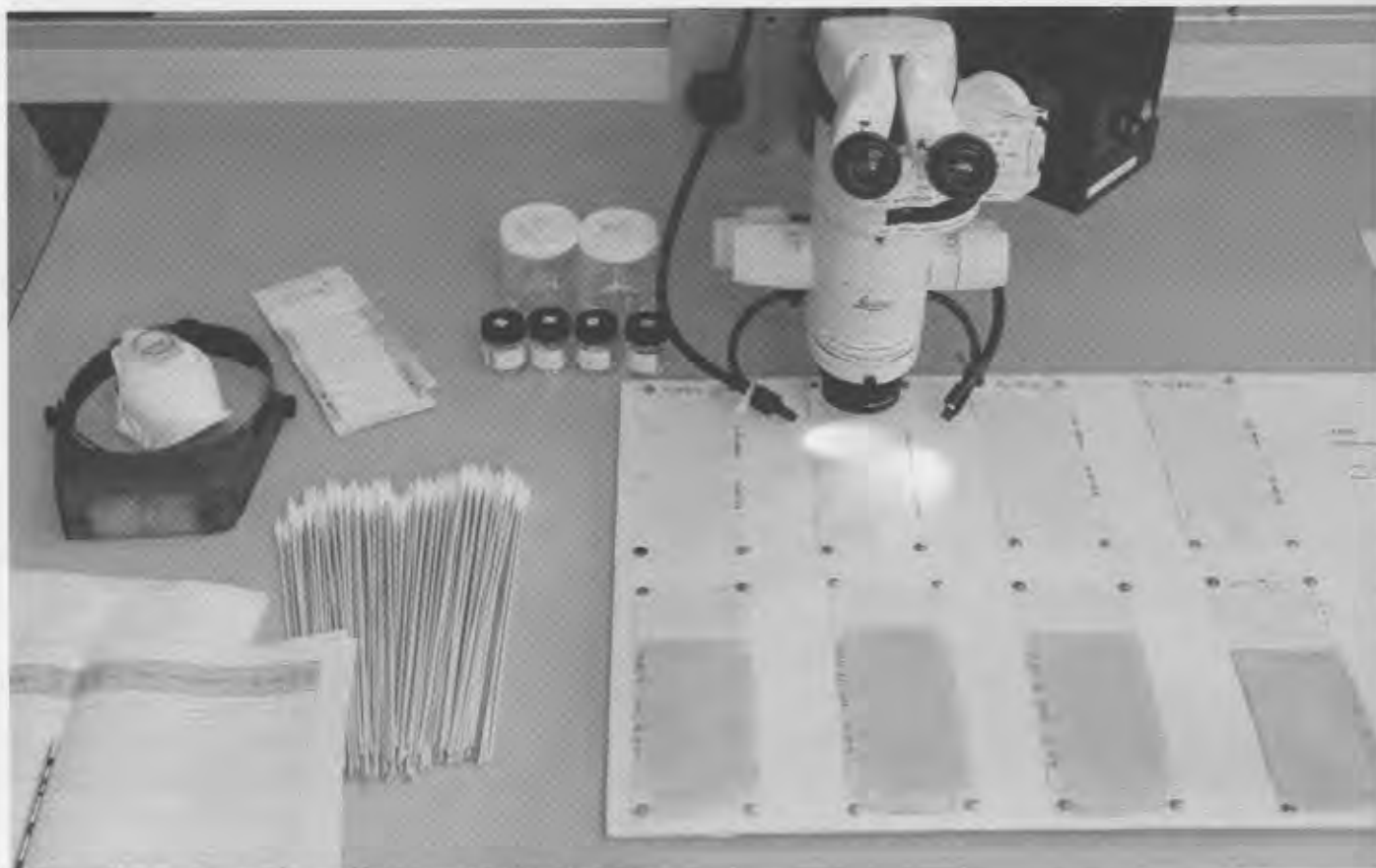
Figure 1: Testing setup with acrylic paint samples for CAPS research.
